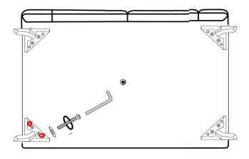
clockwise turning of Allen key for tighten of bolt
